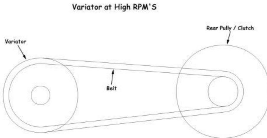
Fig. 2: final stage of CVT. Note that the Variator in this image is the same as the primary clutch and the rear pully/clutch is the same as the secondary clutch
