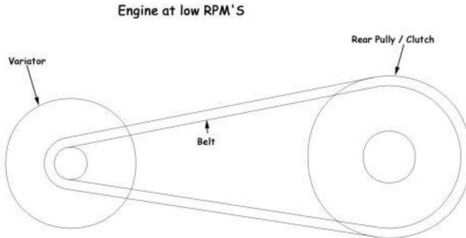
Fig. 1: initial stage of CVT. Note that the Variator in this image is the same as the primary clutch and the rear pully/clutch is the same as the secondary clutch
