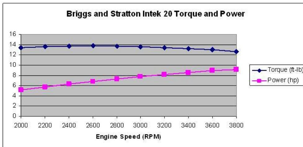
Fig. 4: Power and Torque curves for the Briggs and Stratton Model 20 Engine
